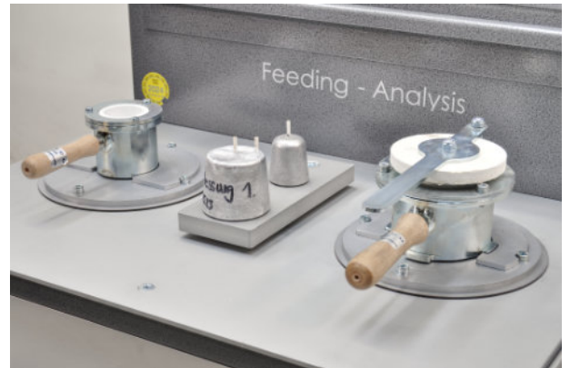
The device combines Thermo-Analysis and Feeding-Analysis
